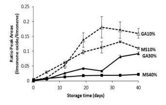
Figure 2. The influence of infeed solids during spray drying on the oxidation of limonene during storage (MS is modified starch; GA is gum acacia; the % shown is the infeed carrier concentration during spray drying).
