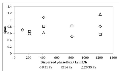
Figure 2. Effect of dispersed phase flux and shear stress on the median particle diameter
