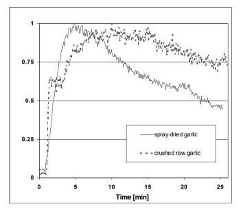
Figure 2: Garlic release from spray-dried encapsulates or crushed raw garlic in water at 80°C as measured by PTR-MS. The maximal response was set at 1.
