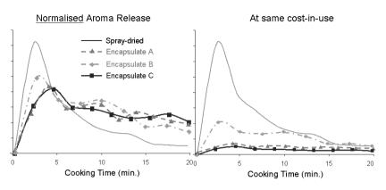
Figure 4: Flavour release from spray-dried and commercial encapsulates in water at 80°C as measured by PTR-MS. The release curves were normalized as such that the area under the curve was the same for each sample. The left picture shows the results at equal flavour load, and the right picture shows the results at equal costs. These data were kindly provided by our colleagues S. Coïc and D. Taal.
