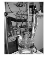
Figure 1: Set up for controlled aroma release measurement of encapsulates by PTR-MS.
